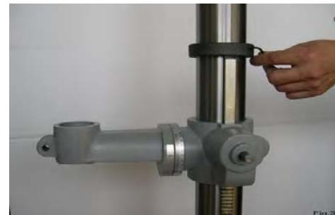
**3. Install bracket handle and clamp bolt. Fig. 4, 5.**
