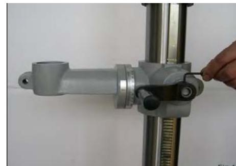
Install clamp bolt to fix table bracket.
