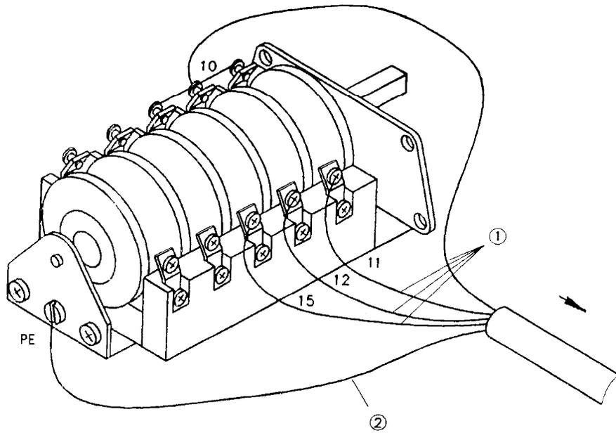
1.....The Cord from the Wiring Board (part no. ZX-XT2)
