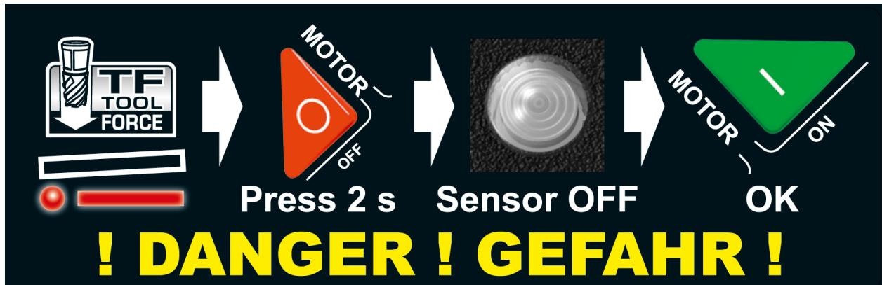
Depending on the version of your core drilling machine it is possible to momentarily deactivate the sensor and its safety appliance.
