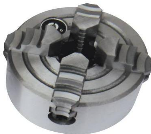
Figure 8-6: Four jaw independent chuck
