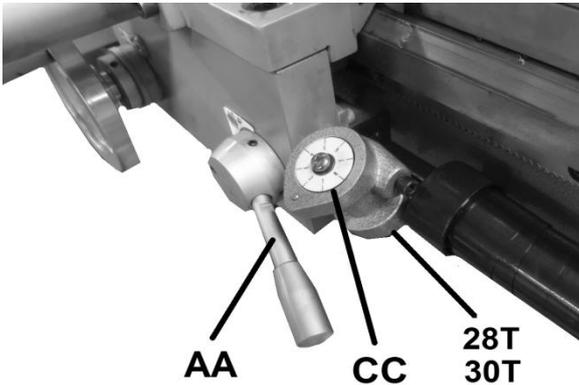
Figure 10-8: Threading Dial
