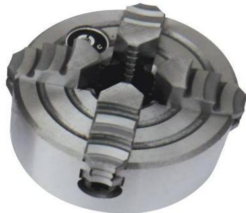
Figure 8-6: Four jaw independent chuck
