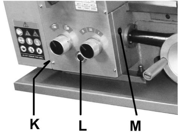
Figure 11-1: Gearbox oil fill-up
