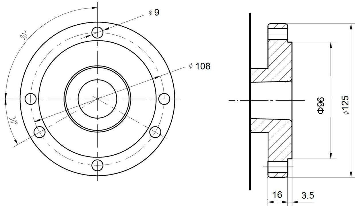
Figure 4-1: Spindle nose mounting
