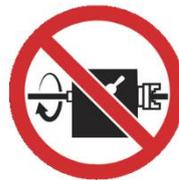
Any work piece stock extending the rear end of the headstock must be covered on its entire length. High danger of injury
