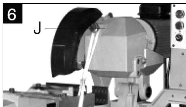
Turn the control handle (L) with trigger switch (K) into the threaded hole (J) and secure with nut in correct position.
