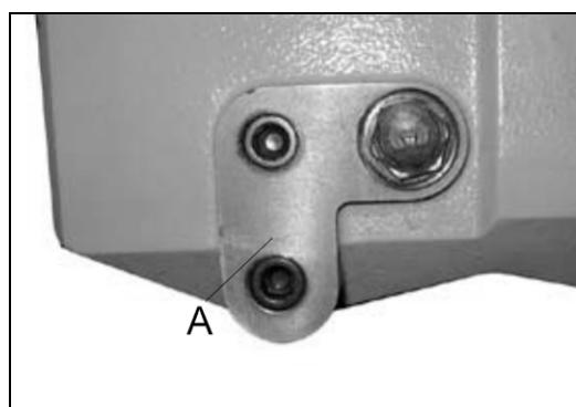
The gear box oil has to be changed periodically. The first oil change is to be carried out after 6 months, and then after that once a year.
