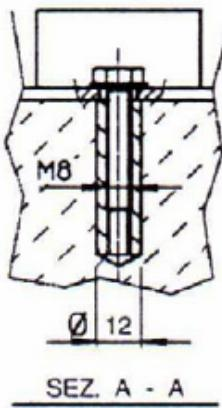
Position the machine on a firm and level concrete floor. Maintain a minimum distance of 800mm from the wall to rear of the machine. Anchor the machine to the ground, as shown in the diagram, using screws and expansion plugs or sunken tie rods that connect through holes in the base of the stand. Ensuring that it is sitting level (see picture).
