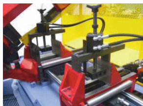
Serrage Vertical Hydraulique
