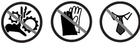
Before operating the machine, remove tie, rings, watches, other jewellery, and roll up sleeves above the elbows.
