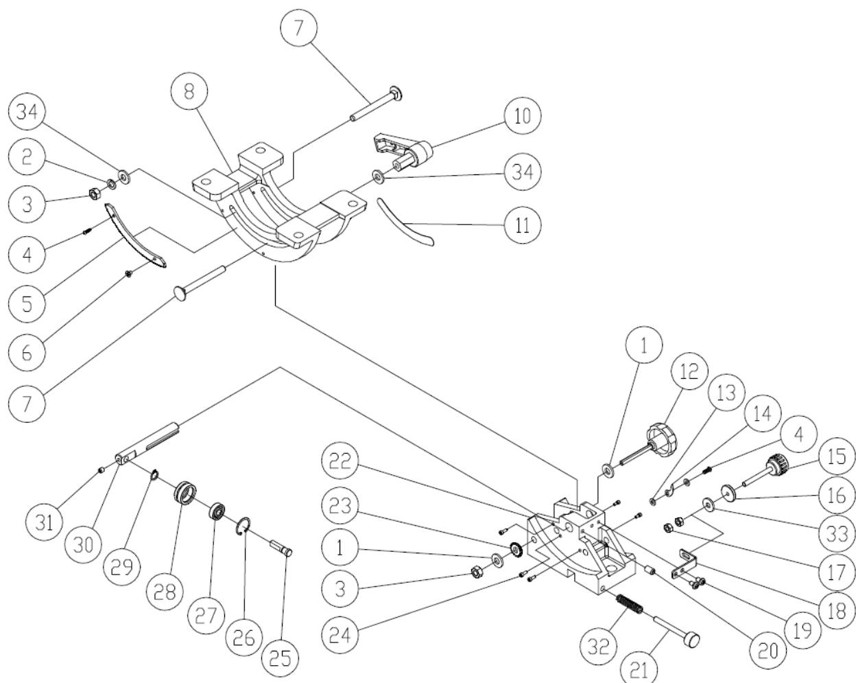
**PART LIST / ERSATZTEILLISTE / LISTE DES PIÈCES DÉTACHÉES****JWBS-15 / JWBS-18 / JWBS-20****Trunnion Support Bracket Assembly**
