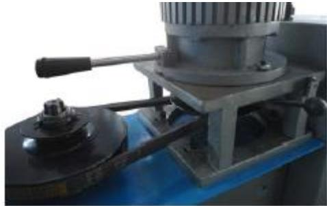
3. Slide the motor toward the pulley.
