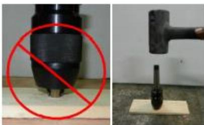
3. Slide the assembled drill chuck and arbor into spindle taper, and slightly hit them by rubber hammer to fit in.
