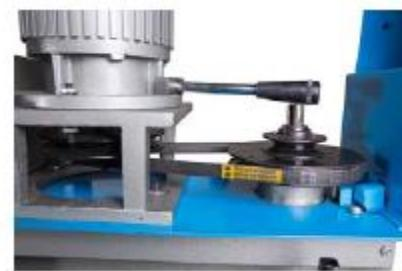
7. Tension should be loose enough to allow 5-10mm movement when pushing the belt from the side.
