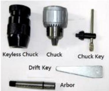
1. Clean the drill chuck, arbor and spindle taper thoroughly before installation. Any insufficient cleaning on mating surfaces may cause drill loosen as operating and unsafe conditions.
