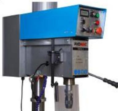
This clear plastic shield should be used whenever conducting a drilling or tapping operation. Clean the safety guard periodically to provide a clear view of the work piece. Adjustments can be done as follows.
