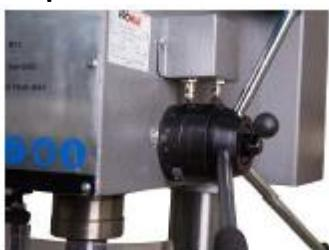
A drilling depth indicator is provided on the side of the drill head. The indicator can be set for depths up to 12.5 cm. The lock knob is provided at the side, on the top of quill lever. Before starting the motor:
