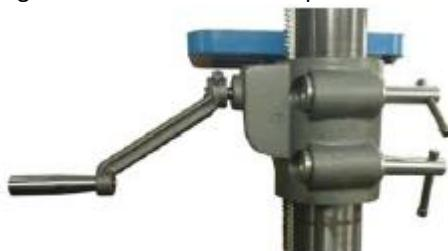
To tilt the table, loosen the lock-lever first to adjust the table to desired angle, then lock the table in position.
