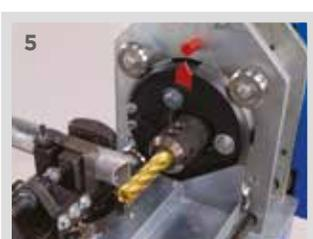
SET TO DESIRED OD. TURN HAND WHEEL COUNTER CLOCK-WISE. ONE REVOLUTION PER WELD JOINT WITH OUT THE NEED TO CHANGE END MILLS REGARDLESS OF THE NOTCH SIZE.
