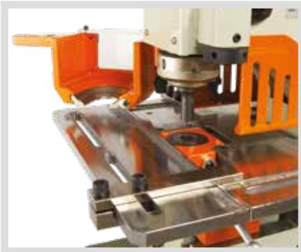
SWING AWAY STRIPPER FOR EASY ACCESS AND FAST TOOLING CHANGES.
