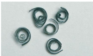
: Moderate chip curling indicates correct cutting conditions
