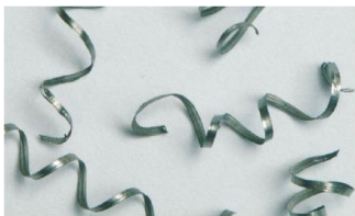
: Large, tightly coiled chips or chips with a bluish tinge indicate excessive feed
